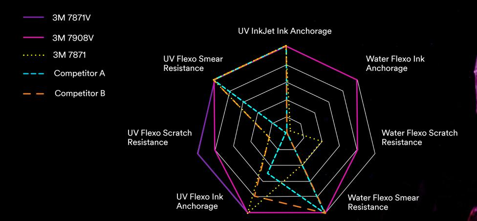
Ink anchorage tested via ASTM 3359 for cross hatch adhesion using 3M™ Scotch Cellophane Film Tape 610. Scratch and smear resistance tested via industry-recognized qualitative tests using thumbnail scratch and thumb pressure smear. For more information, please contact a 3M expert at 3M.com/durablelabels.
